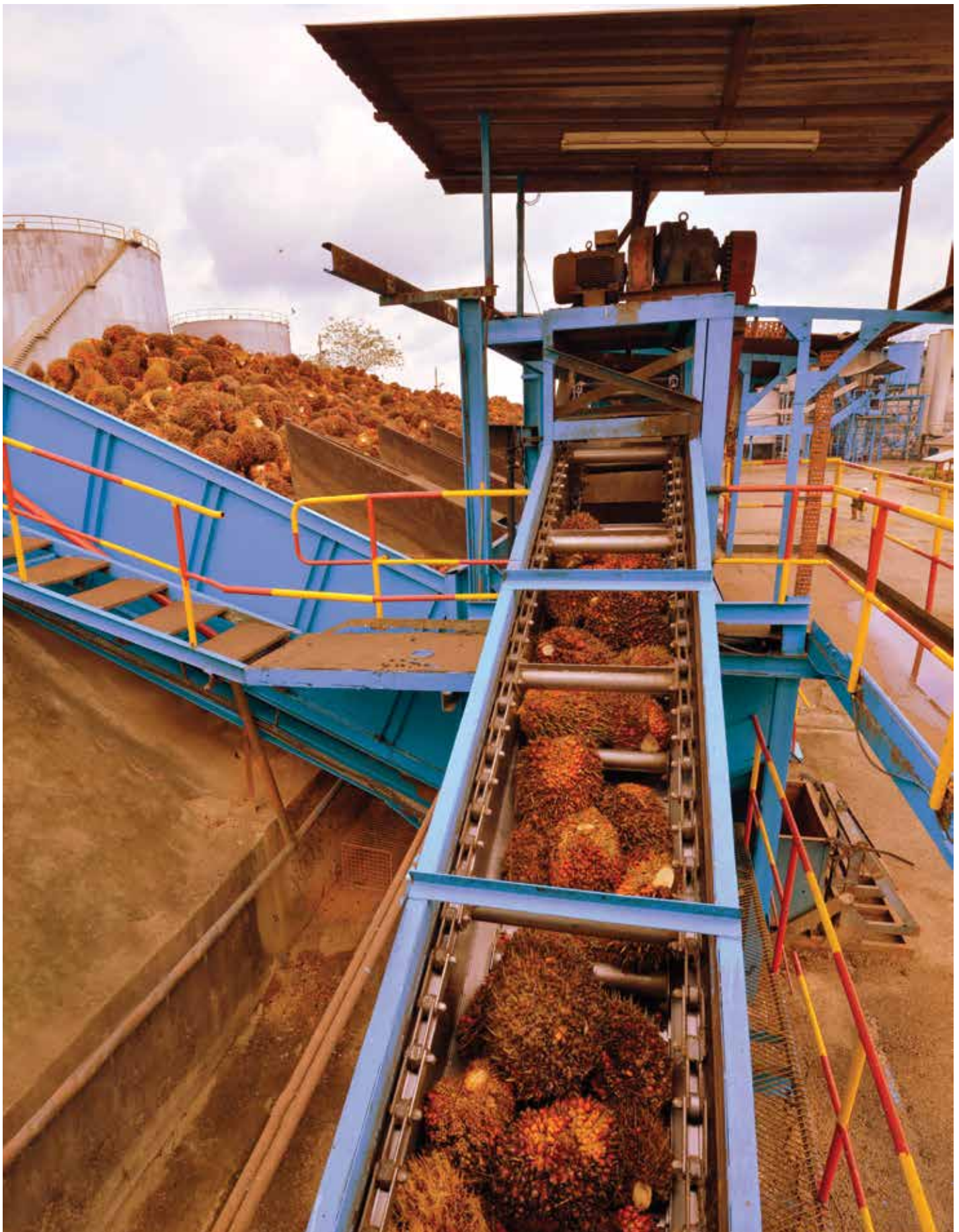
60 tonnes per hour; Tereh Palm Oil Mill, Kluang, produced 68,000 mt CPO and 19,000 mt PKO in 2017
